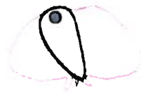
Figure 4. T310d 2.4GHz Elevation Antenna Pattern
