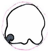
Figure 2. T310d 2.4GHz Azimuth Antenna Patterns
