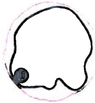
Figure 2. T310d 2.4GHz Azimuth Antenna Patterns
