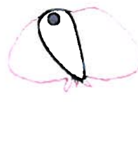
Figure 4. T310d 2.4GHz Elevation Antenna Patterns
