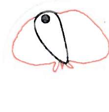
Figure 4. T310d 2.4GHz Elevation Antenna Patterns
