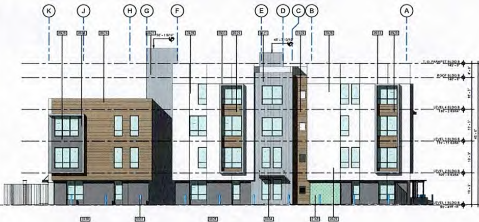
2 EAST ELEVATION - BLDG B 1/8" = 1'-0"
