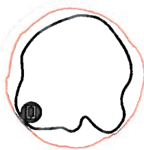
Figure 2. T310d 2.4GHz Azimuth Antenna Patterns
