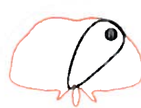
Figure 5. T310d 5GHz Elevation Antenna Patterns
