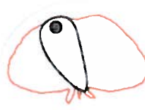
Figure 4. T310d 2.4GHz Elevation Antenna Patterns
