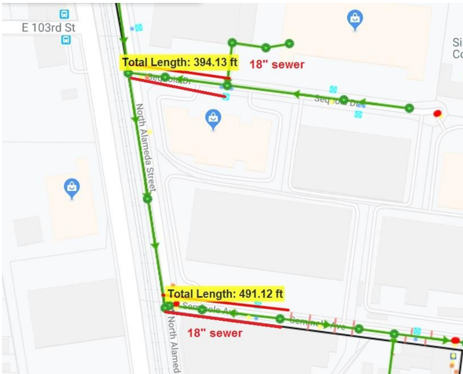
Figure 4-12: Sequoia Drive and Seminole Avenue Pipeline Replacements
