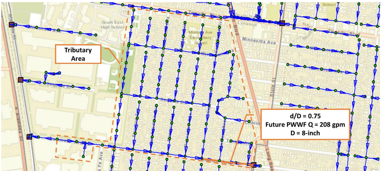
Figure 4-8: d/D > 0.5 Pipeline – Seminole Avenue & State Street
