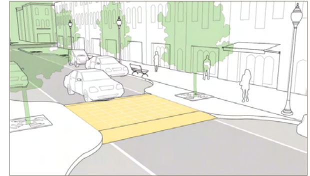
NACTO Speed Table Diagram. The feature shown in yellow is a table top crossing, also called a speed table, to facilitate a better pedestrian crossing experience and serve as a vehicular speed calming device. They are often used in conjunction with curb extensions as shown. Image Credit: Urban Street Design Guide, National Association of City Transportation Officials (NACTO)
