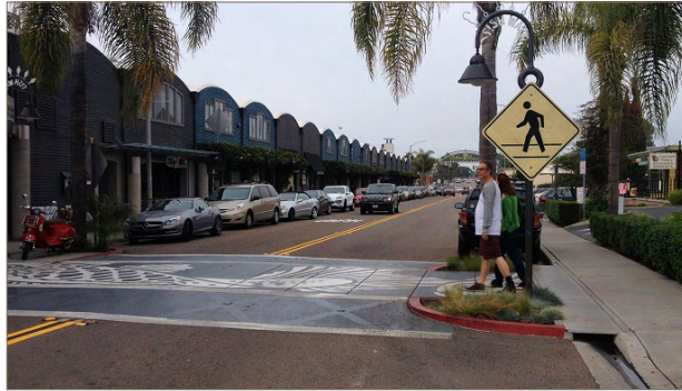
Cedros Avenue, Solana Beach, CA. Curb extensions and a graphic crosswalk design help drivers and pedestrians alike at mid-block crossings.
